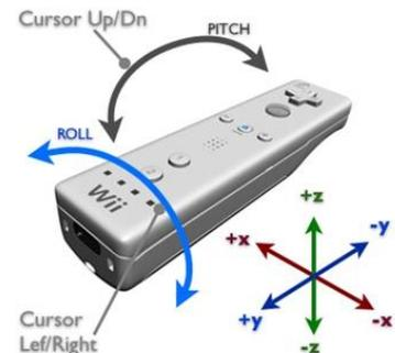
In MOUSE MODE the ⊖ and ⊕ buttons are the mouse buttons.
